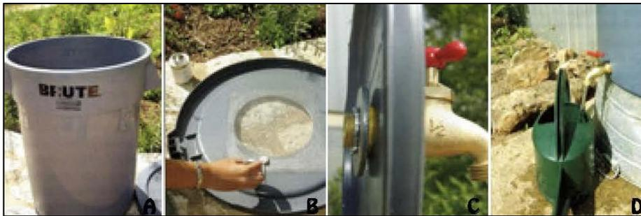
Figure 2. A) A common, heavy-duty garbage can; B) Preparing the lid; C) Preparing the faucet assembly; D) Completed rain barrel.
