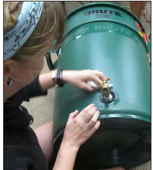
Figure 3. Insert the faucet assembly and wipe off excess silicone from the rubber washer.
