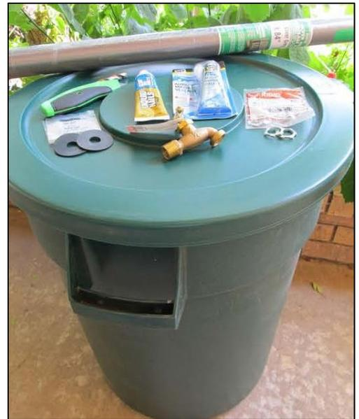
Figure 1. Parts and tools necessary to build a homemade rain barrel.
