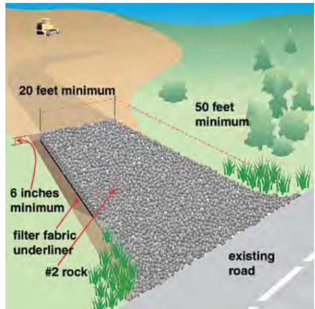
Figure 4. Stabilized construction exit.
